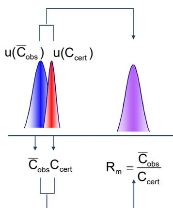
$$\frac{u(R_m)}{R_m} = \sqrt{\left(\frac{u(\bar{C}_{obs})}{\bar{C}_{obs}}\right)^2 + \left(\frac{u(C_{cert})}{C_{cert}}\right)^2}$$
