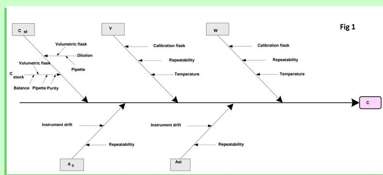
The sources of uncertainty for the method were identified by constructing a cause-and-effect diagram. The "effect" is the result of the analysis, the "cause" is the main parameters controlling the result. The relationship between the result (or the "measurand") and the parameters (or the "input quantities") are shown in Eq. (1) and the cause-and-effect diagram are shown in Fig. (1).
