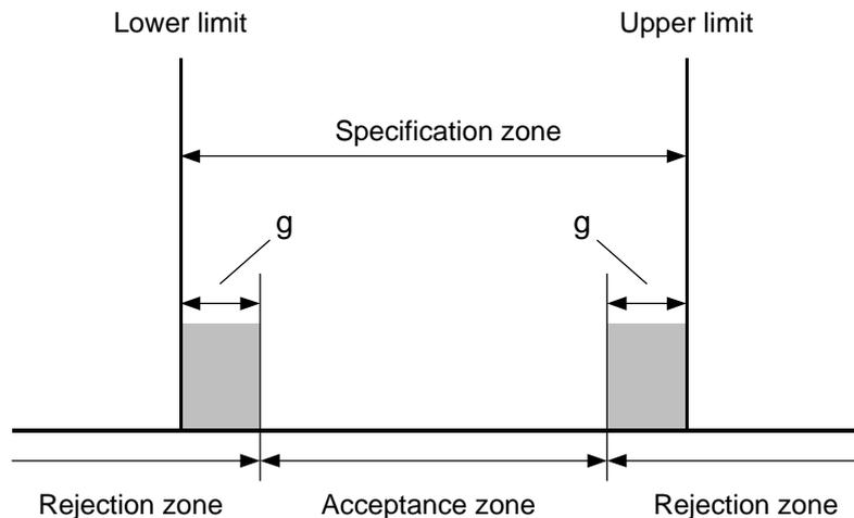
The figure shows the relative positions of the specified limits and of the acceptance and rejection zones for low risk of false acceptance.
