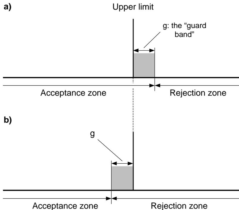
The figure shows the relative positions of the acceptance and rejection zones for a) high confidence of correct rejection; b) high confidence of correct acceptance. The distance  $g$  is often called the ‘guard band’.
