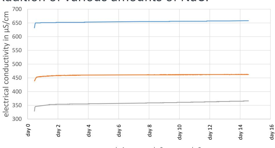
The slight increase over time is probably due to the bleeding of the pH electrode
